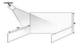
500-WATT AND 1000-WATT QUARTZ SPOTLIGHT INSTALLED OVERHEAD IN CEILING, THESE UNITS WORK WILL FOR LIGHTING SPECIFIC MACHINERY.
